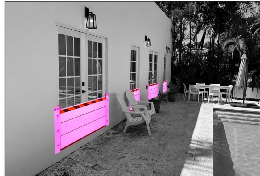
Figure 1B. Rendering of proposed conditions (Alternative A implemented). Temporary barriers for openings installed.
