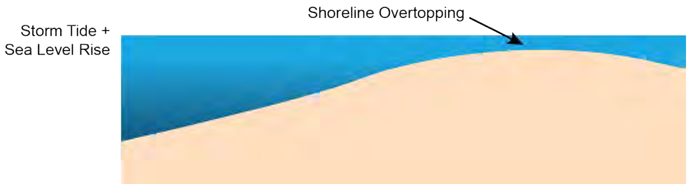
Figure D.6: Conceptual shoreline cross section illustrating overtopping.
