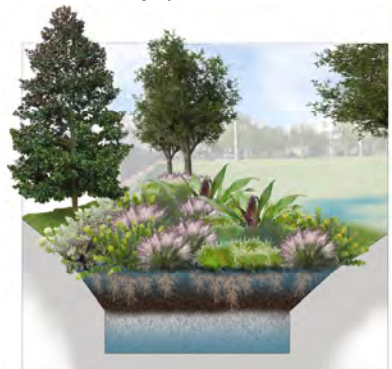
Typical bioretention cross-section with surface depression, Florida-friendly plants, engineered soil, and gravel layer
