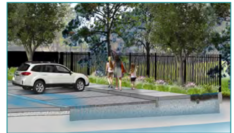
Typical cross-section for subsurface infiltration/storage system filled with gravel
