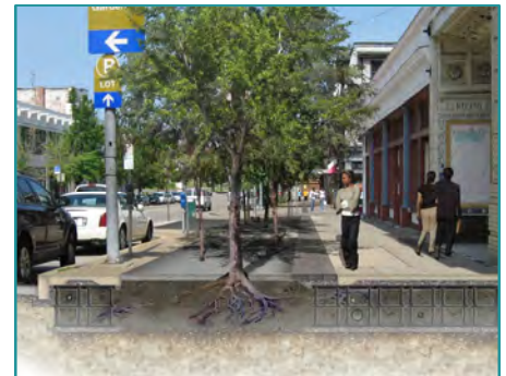
Typical enhanced tree trench section using suspended pavement system/modular soil cells (Source: Viridian Landscape Studio)
