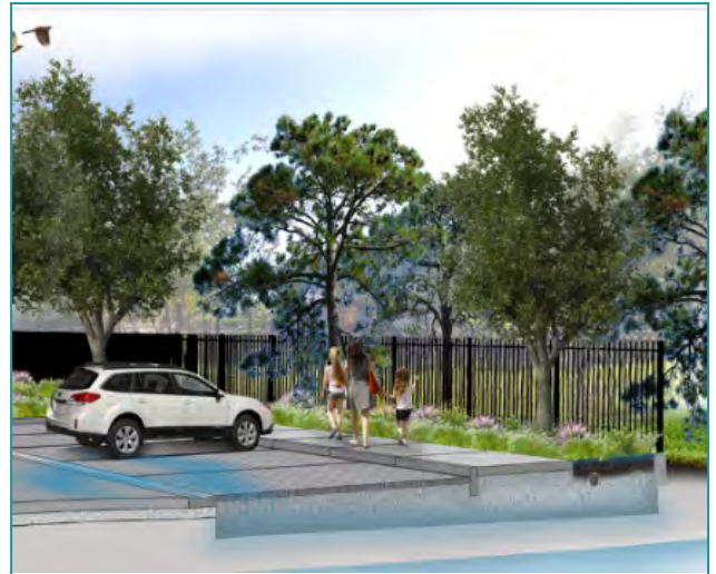
Permeable pavement, bioswale, and subsurface infiltration next to a park
