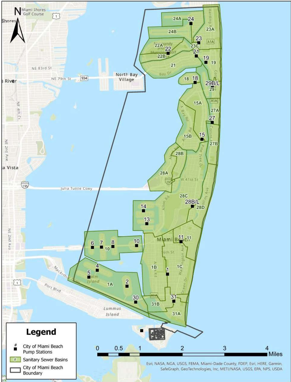
Figure 1-1: Sewer Service Area & Basin Locations
