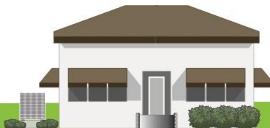
Flood Protection (Dry Flood Proofing)
