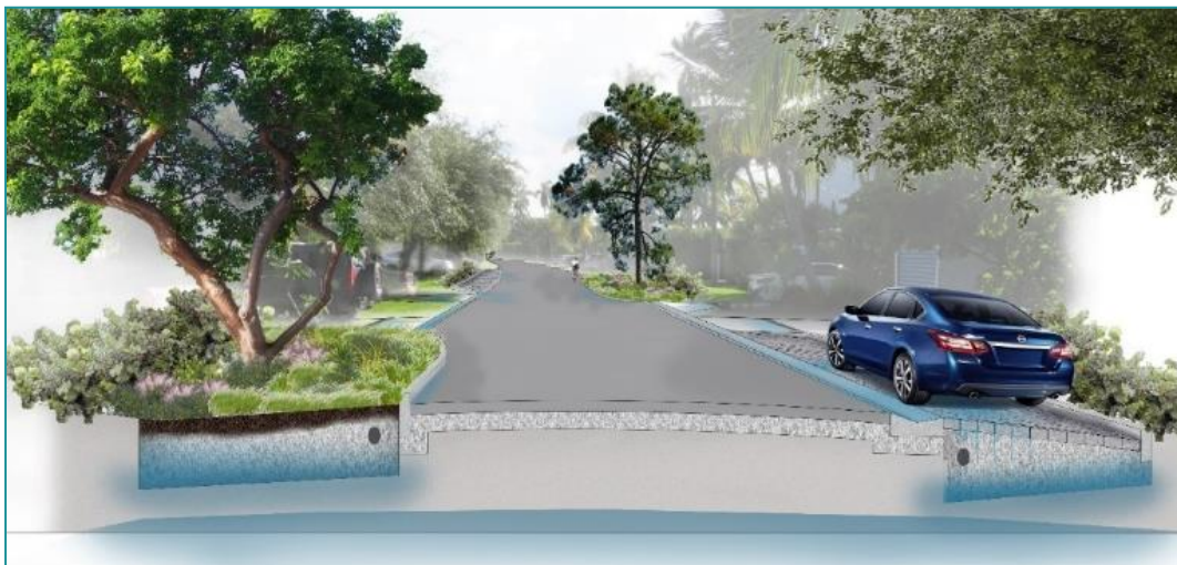
A rendering of bioretention and permeable pavement on a typical residential street in Miami Beach
