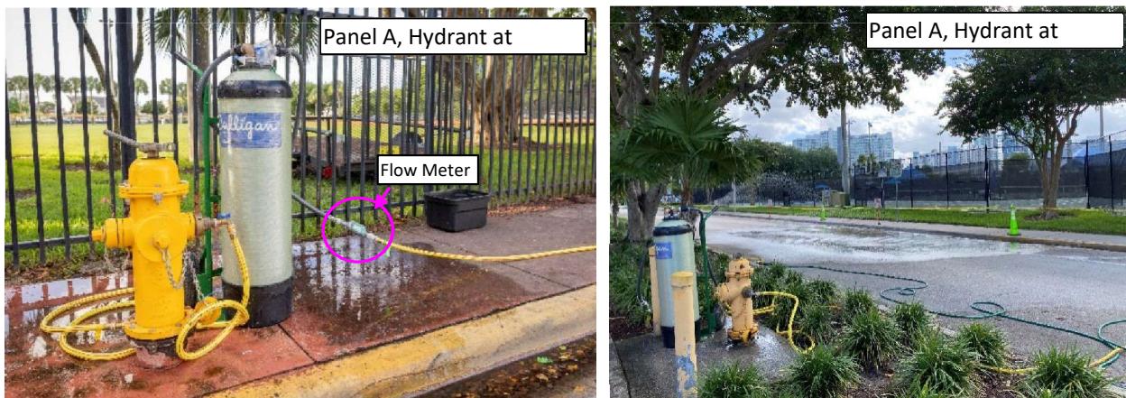
Figure II.3. Hydrant set up for experimentation showing the chlorine filter downstream of the hydrant at Carlyle (Panel A) and at Byron (Panel B). Panel A also shows the flow meter used to measure flow from the filter system.
