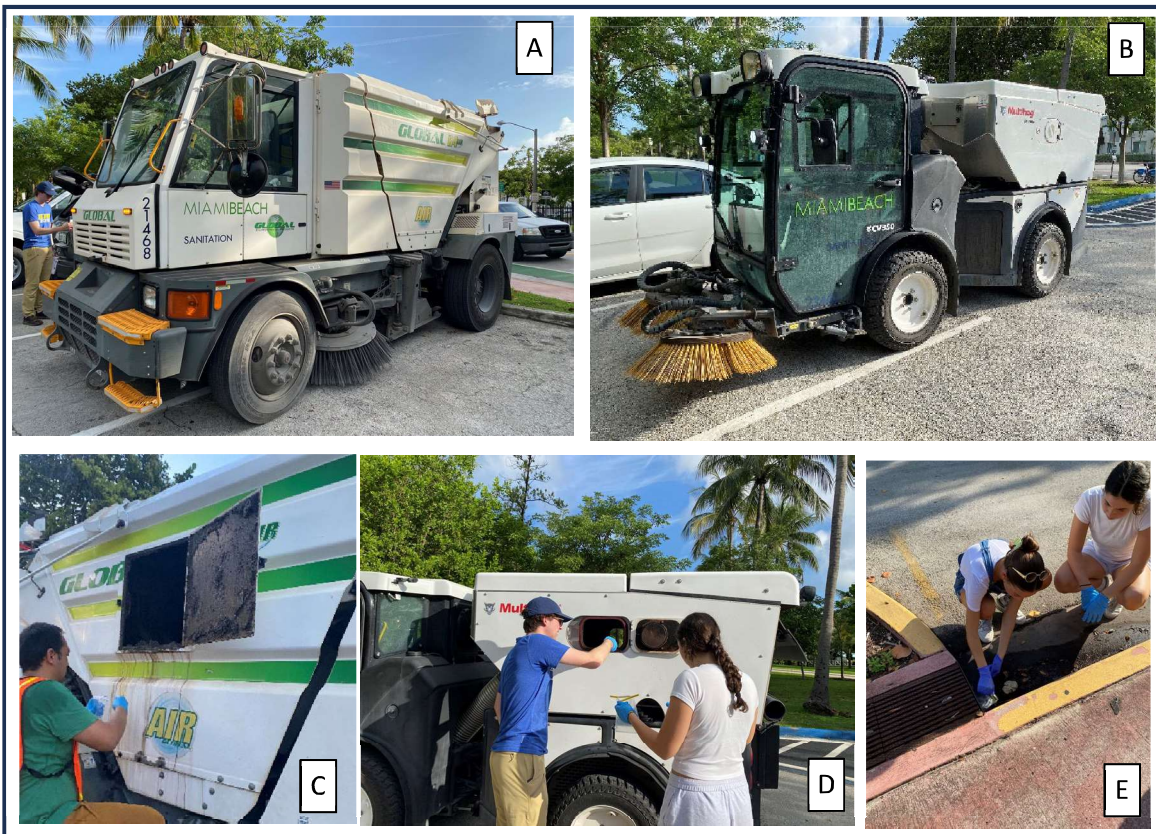
Figure II.8. Photos from street sweeper and sediment sample collection. Large industrial street sweeper (panel A), small industrial street sweeper (panel B), sample collection from large street sweeper (panel C), sample collection from small street sweeper (panel D), Sample collection from curb at Dickens (panel E).
