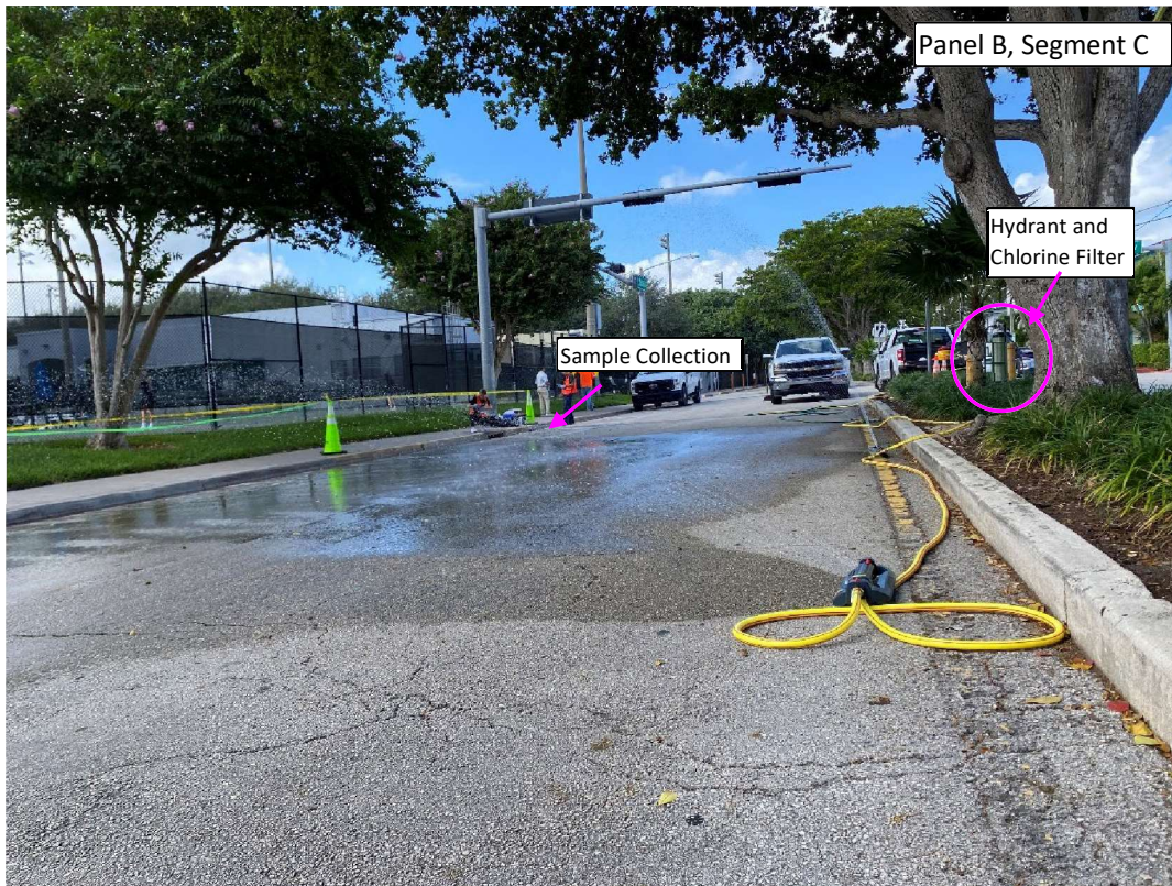
Figure II.4. Examples of street sprinkler set up for Segment A (Panel A) and for Segment C (Panel B). Three lawn sprinklers were used at each segment with sample collection in the stormwater gutter downstream.
